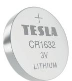
**DESCRIPTION:** Mercury Free Lithium Cell Battery, CR1632 / Non-Rechargeable **CHEMICAL SYSTEM:** Lithium Manganese Dioxide SHELF LIFE: 7 years **NOMINAL VOLTAGE:** 3 Volts **NOMINAL DIMENSIONS:** Ø 16 mm × 3.2 mm **APPLICATIONS:** Suitable for flashlights, car keys, watches, scanners etc. **STORAGE TEMPERATURE:** +10 °C to + 25 °C Should be stored in dry and cool place. **NOMINAL WEIGHT:**
